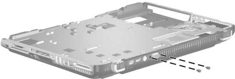
Hex Socket HM5.0×9.0 Screw Lock Locations
