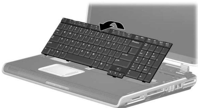
Removing the Keyboard
